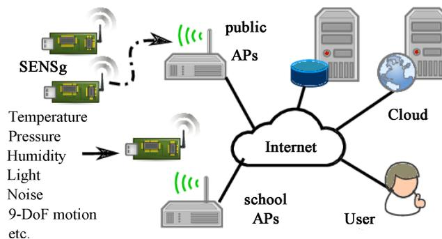
**Figure 1.** SENSg Architecture.
