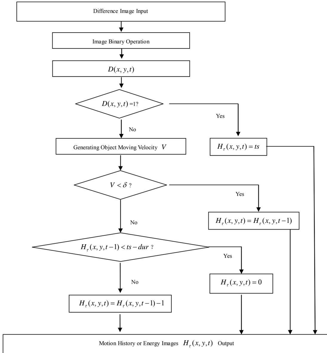
Figure 2. MHoEI algorithm flow chart.
