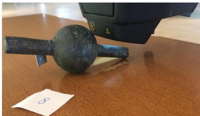
**Figure 12.** ELIO XRF portable system acquiring fluorescence spectrum from the ball bearing n.8.
