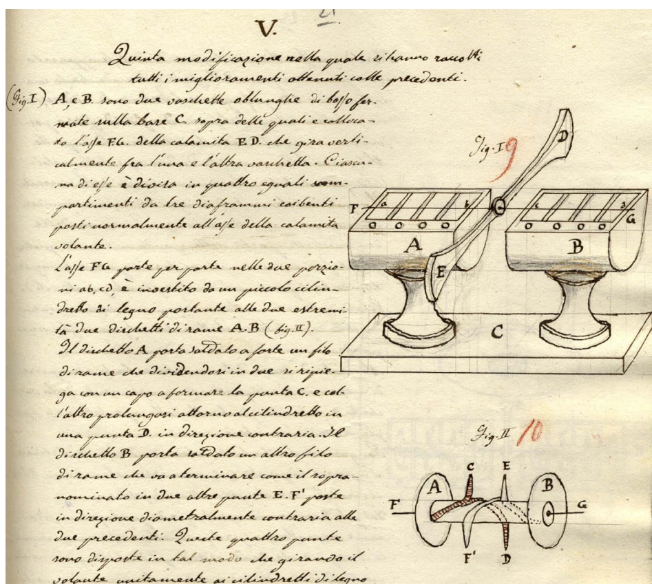
Figure 5. The original drawing of the last commutator-interrupter as modified by Vincenzo Vignola and found in Paolo Vignola's manuscript memoir. By courtesy of "Accademia di Agricoltura, Scienze e Lettere" in Verona.
