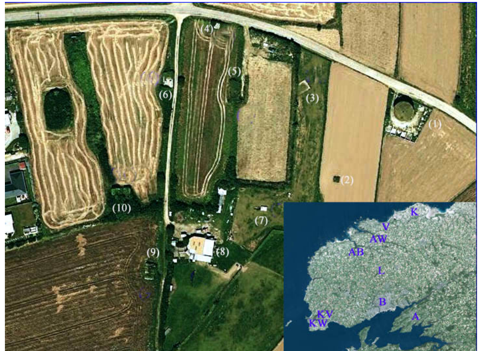
Figure 1. Keringar Vihan radar base-(1) water reservoir tank, (2) bunker of unknown type and purpose, (3) bunker of unknown type and purpose, (4) bunker of unknown type and purpose at the entrance of the base, (5) bunker of unknown type, probably either troop lodgment, or Flak fire control bunker, or a bunker type I406A for permanent machinery like power generators, (6) Flak bunker, (7) bunker of unknown type and purpose, (8) type 1 split wall emplacement for radar Freya , (9) Flak bunker, (10) type 5 brick, split wall version for radar Freya A Armorique peninsula, AB Aber Benoît, AW Aber Wrach, B Brest, K Kervinagam-Kerdené radar base; KV Keringar Wraz M. K. B Graf Spee, KV Keringar Vihan radar base, V Vougo-Kerizoc radar base, L Lesneven [Geoportail].
