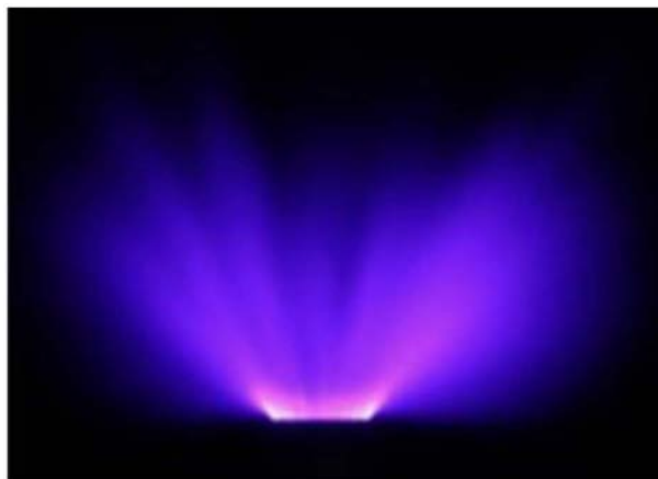
Figure 8. A light from corona discharge or ionization that appears when the electric field exceeds about 3000 Volts/mm in the air (Courtesy of Tao Shao, et al. 2011 “Runaway electrons and x-rays from a corona discharge in atmospheric pressure air” New Journal of Physics , Volume 13, Nov 2011).
