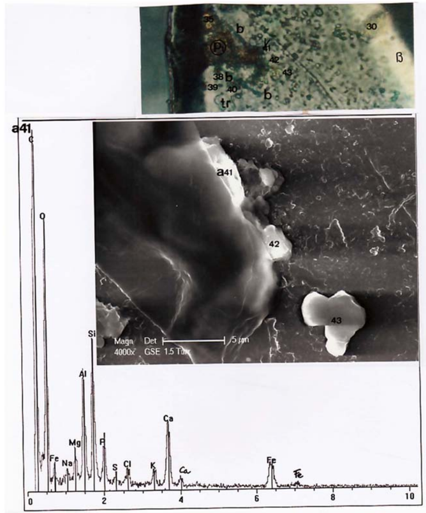
Figure 6. The a41 particle. Above photograph: optical view (1200×) of the left part of the low A area, showing the a41 particle (arrow point). P1 is a triangular fold of PVC plastic in this area part (B is the right border of the A area). Below photograph: SEM1 photograph (4000×) in GSE, showing the emerging part of the a41 particle (a42 is a glass and a43 a trilobed calcium carbonate). Below: the HR a41 spectrum. C: carbon; O: oxygen; Fe (three peaks): iron; Na: sodium; Mg: magnesium; Al: aluminium; Si: silicium; P: phosphorous; S: sulphur; K: potassium; Ca (two peaks): calcium.
