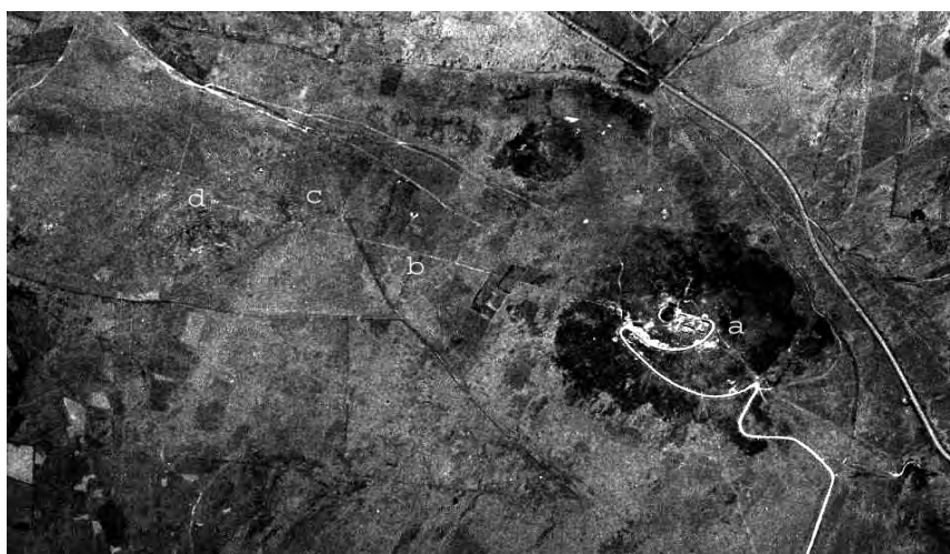
Figure 2. Be-2 site—(a) Mont Saint-Michel de Brasparts; (b) Cable trench; (c) Stone straight alignment; (d) Monitoring mast concrete support.
