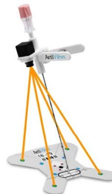
Figure 2. The miniature video camera is mounted on the instrument and captures the fiducial markers that allows for instrument tracking in CT space.
