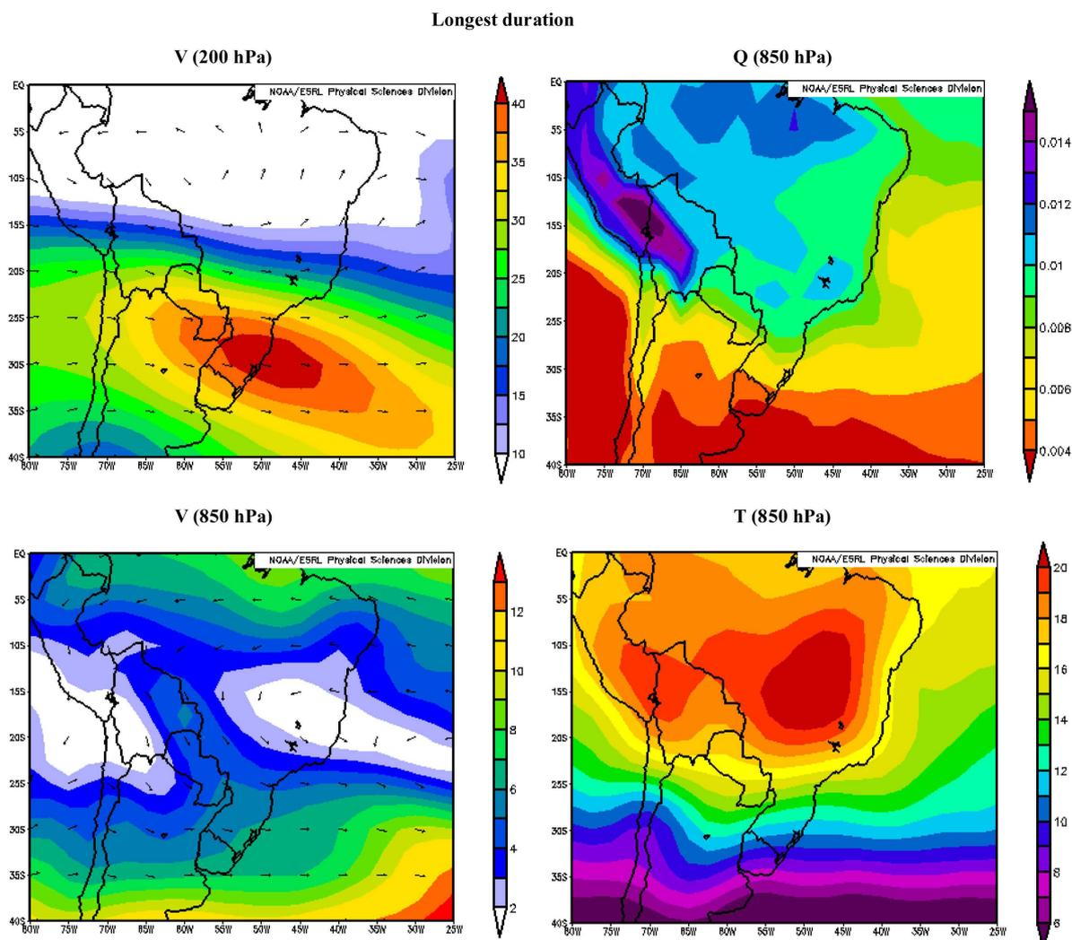
**Figure 15.** Composite mean fields of 200-hPa and 850-hPa winds ( $\text{m}\cdot\text{s}^{-1}$ ), 850-hPa specific humidity ( $\text{kg}\cdot\text{kg}^{-1}$ ) and temperature ( $^{\circ}\text{C}$ ) for the 10 longest span systems starting at the Andes Mountains.
