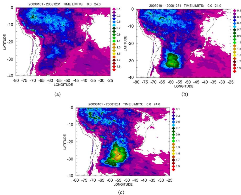
**Figure 18.** Average rainfall fields (mm) for all organized convection systems starting at Andes Mountain range between 2003 and 2008 with spans of 300 km to 700 km (a), 701 km to 1700 km (b) and 1701 km to 3700 km (c) corresponding to 210, 144 and 82 episodes, respectively.
