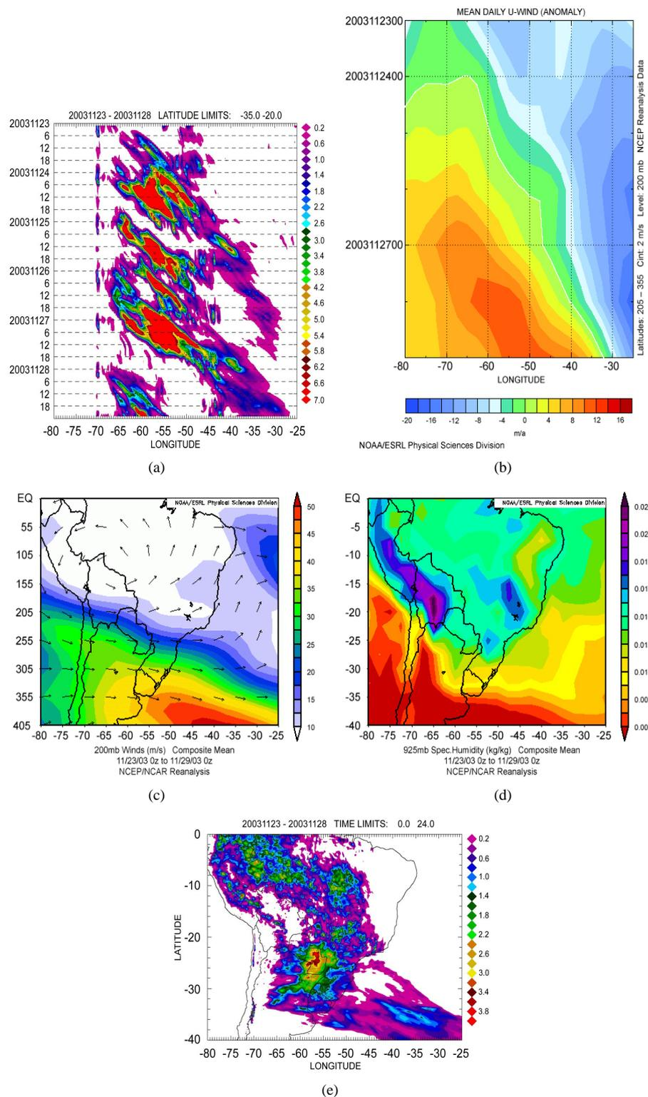
**Figure 10.** Episodes of organized convection between 23 and 29 November 2003. It shows Hovmöller diagrams of one-hour rainfall accumulation average (a) and 200-hPa zonal wind anomalies (b); the average 200-hPa wind field (c), average 925-hPa specific humidity (d) and the resulting rainfall accumulation (e). Longitudes, latitudes, geographic contours, color scale are indicated.
