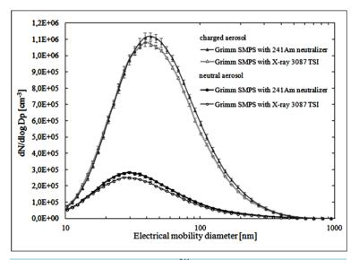
Figure 2. Aerosol size distribution for <sup>241</sup>Am and X-ray neutralizers (charged and neutral particles).
