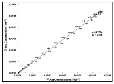
**Figure 5.** Particle concentration correlation between SMPS spectrometer data taken with the X-ray model 3087 TSI and the <sup>241</sup>Am neutralizers.
