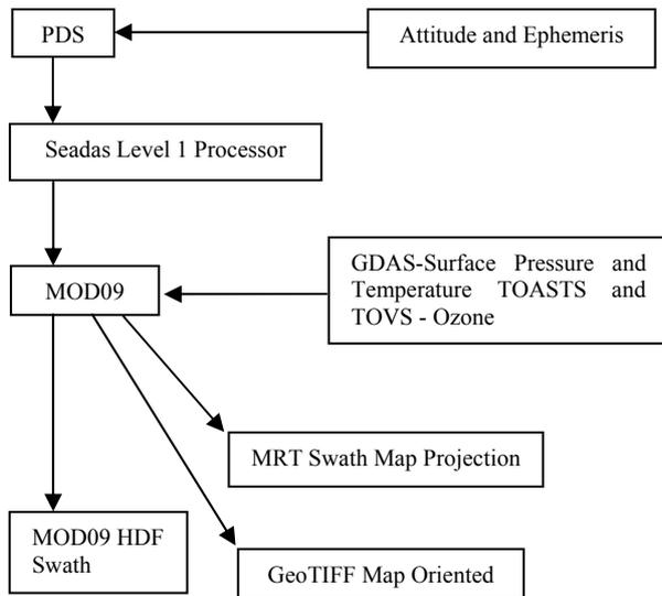
**Figure 2. MOD09 Atmospheric correction process work flow to generate a full single swath at ACRES, Australia.**
