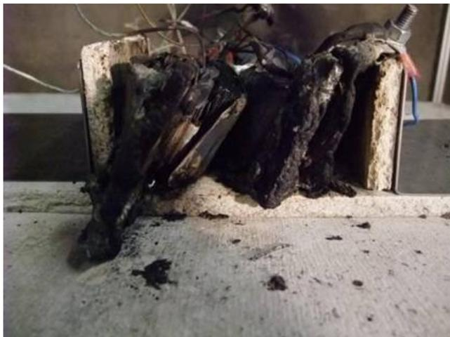
**Figure 11.** Module of 4 cells after overcharge of a single cell.
