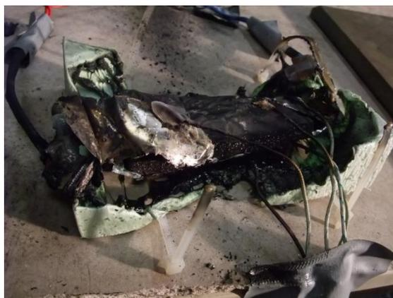
Figure 6. Destroyed overcharge cell after the test, burned and ruptured.
