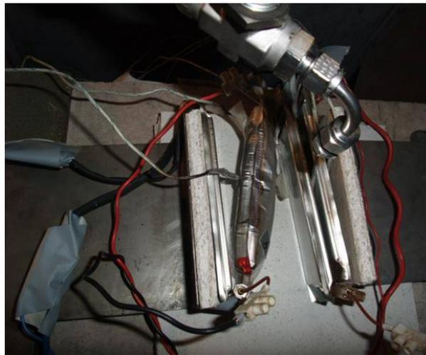
Figure 13. Cell 9 inflated / module with CO<sub>2</sub>-cooling.
