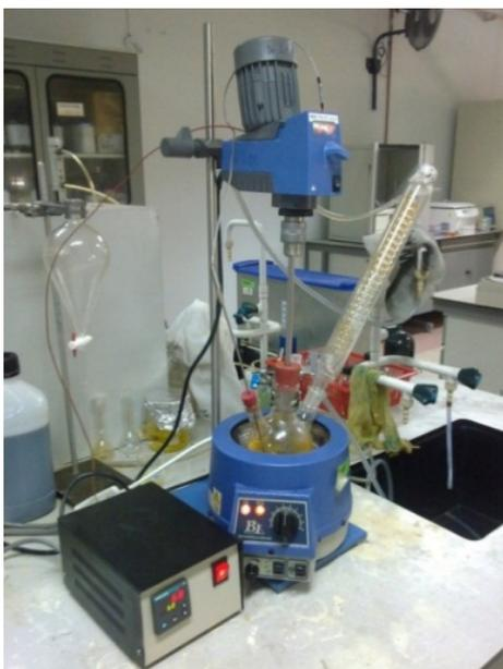
**Figure 1.** Transesterification experimental setup.
