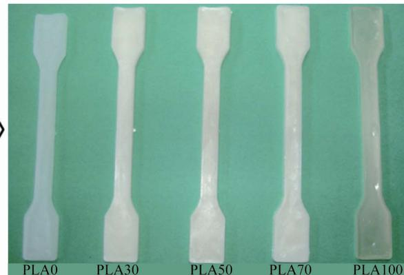
**Figure 5. Injected samples and their processing condition.**
