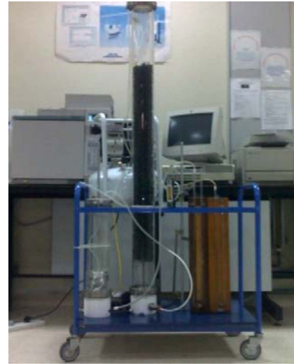
Figure 1. Mobile pilot-biofilter unit.
