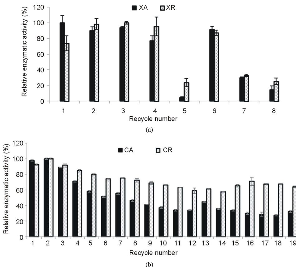
**Figure 2.** Reusability of cellulase and xylanase immobilized by adsorption and reticulation. (a) XA: xylanase immobilized by adsorption; XR: xylanase immobilized by reticulation; (b) CA: cellulase immobilized by adsorption; CR: cellulase immobilized by reticulation. Data were expressed as means of three independent trials. Relative activities were calculated by taking maximum immobilized-enzyme activity as 100% in each case.
