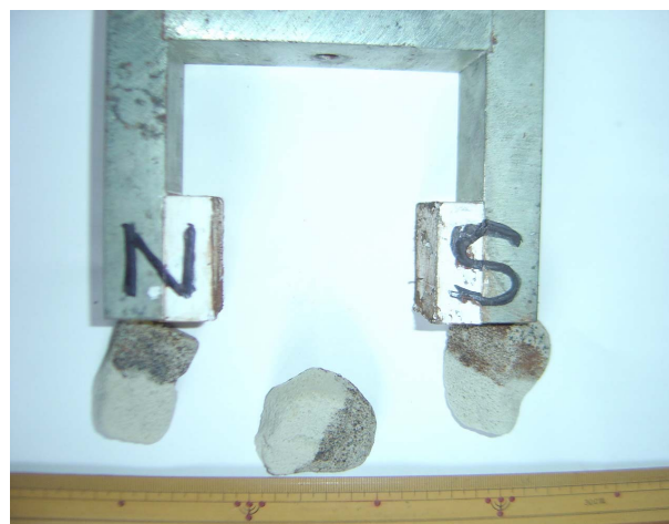
Figure 1. Recovery type of porous ceramic carrier made from waste glass. In the porous ceramic block, one part, shown as black moiety contains 5% iron for recovery by electromagnet (expressed as N and S). Photosynthetic bacterium, Rhodobacter sphaeroides SSI immobilized ceramic was recovered from water, soil and sediment mud using electromagnet after Cs and Sr removal treatment.
