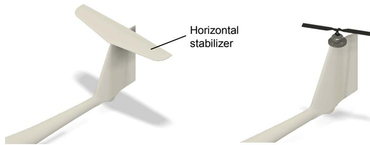
**Figure 1.** The proposed roto-stabilizer as viable substitution for conventional horizontal stabilizer.
