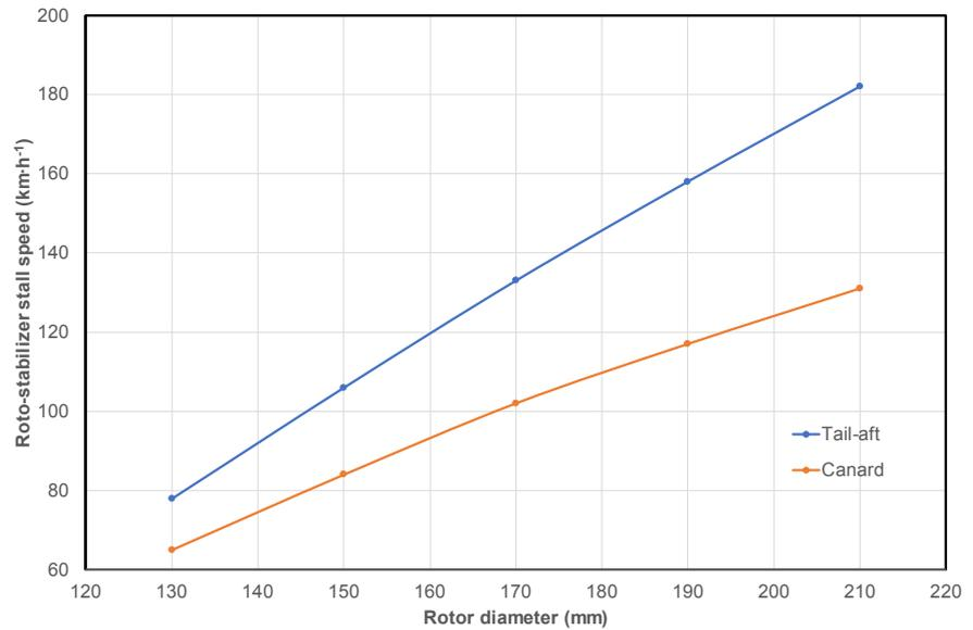
**Figure 5.** The sailplane's airspeed at which the roto-stabilizer's pitch control diminished as a function of its rotor diameter. The wing airfoil was S3021-095-84.
