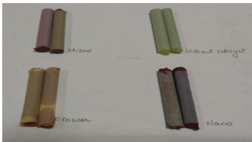
**Figure 3.** Solid propellant strands of various Iron Oxide catalyst.
