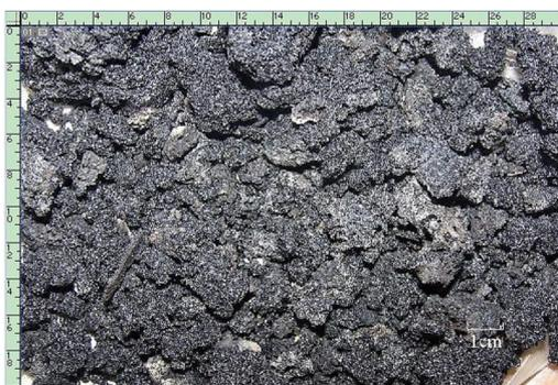
Figure 8. Blockage in the pipeline
