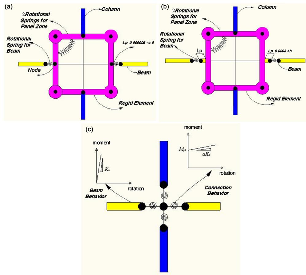
**Figure 2.** Schematic model of panel-zone elements: (a) Panel-Zone element used in pre-Northridge buildings (corresponding to WUF connection for low ductility buildings); (b) Panel-zone element used in post-Northridge buildings (corresponding to RBS connection for high ductility buildings); (c) Schematic connection modeling in the braced frame.
