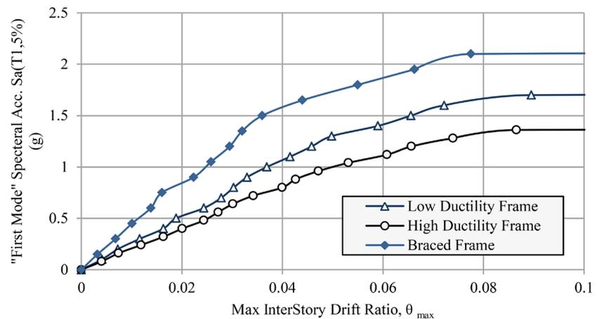
**Figure 7.** Median IDA curves for three frames.
