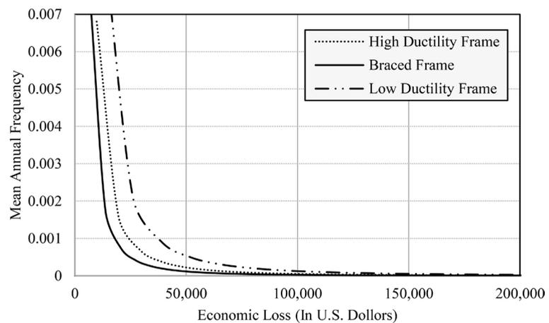
**Figure 10.** Comparing loss curves obtained from three structure.
