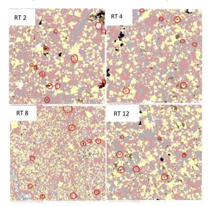
**Figure 1.** Mineral maps generated from electron probe microanalysis of 4 Round Top rhyolite samples. YF grains circled in red, some with multiple YF grains in close proximity. Mineral colors: K-spar (pink), albite (gray), quartz (yellow), magnetite (black) and annite mica (brown) and YF (red and circled). Field of View 2 mm  $\times$  2 mm.
