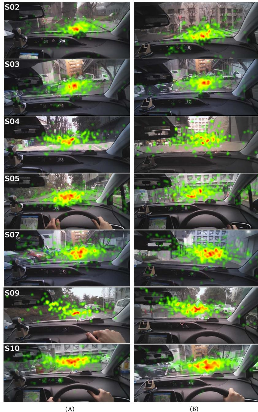
**Figure 7.** Heat map of driver fixation points from seven subjects whilst driving under both conditions. (A) With agent; (B) Without agent.
