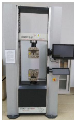
**Figure 4.** Universal test machine.
