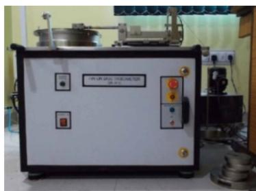
**Figure 3.** Pin on disc tribometer.
