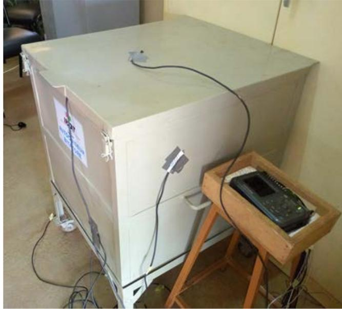
**Figure 3.** Experimental device for the determination of heat losses and time constant.
