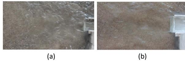
**Figure 3.** The mainstream flow through apron of  $Q = 400.48 \text{ m}^3/\text{s}$  (a), and  $Q = 291.34 \text{ m}^3/\text{s}$  (b).
