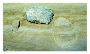
**Figure 4.** Liquefied sand behaving like a "heavy fluid," in which blocks may "swim" (detail from [4]; site: Olivelund).
