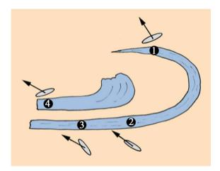
**Figure 18.** In a plastic deformation, sample 1 should have had a reversed paleomagnetic polarity. This is not the case, all four samples have virtually the same polarity. The reason for this must be that the fold structure was formed under fluid conditions; *i.e.* liquefaction [21]. Arrows mark direction of declination. Ellipsoids give direction of the long axis of AMS.
