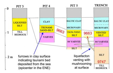
**Figure 16.** In a number of pits and a major trench at Iggesund Harbour [4], we recorded the interaction of strong liquefaction with venting and mushrooming at the surface, and the deposition of a tsunami bed from a wave arriving from the epicentre 12 km to the ENE (as evidenced by marks in the clay surface of Pit 4).
