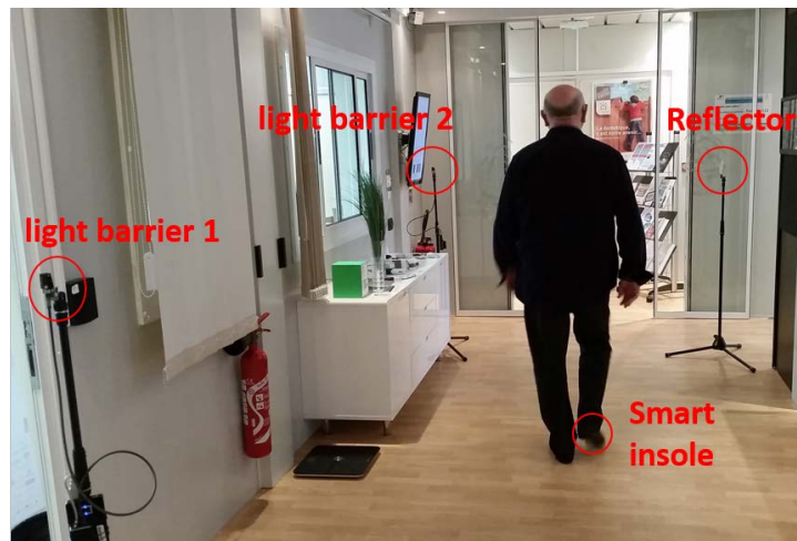
Figure 7. Calibration system with a volunteer.
