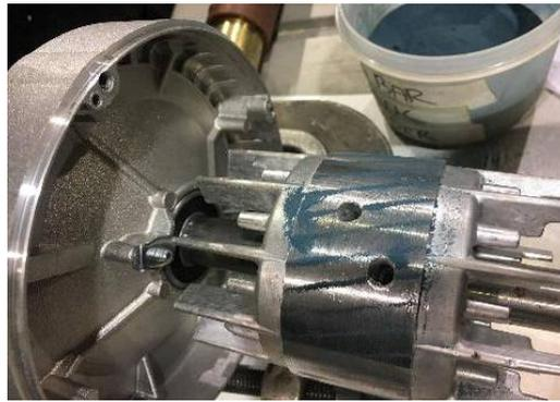
**Figure 3.** An example rotor with two simulated broken rotor bars. The power can help make drilling on the rotor bars.
