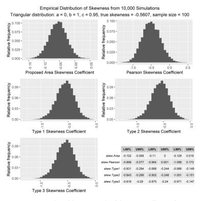
**Figure 19.** Histograms and confidence intervals of skewness coefficients from 10,000 simulations of n = 100 samples from Tr (0, 0.95, 1); standard skewness = -0.56, Pearson skewness = -0.52, area skewness = -0.06.
