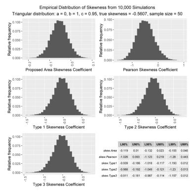
**Figure 17.** Histograms and confidence intervals of skewness coefficients from 10,000 simulations of n = 50 samples from Tr (0, 0.95, 1); standard skewness = -0.56, Pearson skewness = -0.52, area skewness = -0.66.
