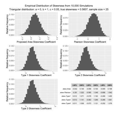
**Figure 20.** Histograms and confidence intervals of skewness coefficients from 10,000 simulations of n = 25 samples from Tr (0, 0.05, 1); standard skewness = 0.56, Pearson skewness = 0.52, area skewness = 0.06.
