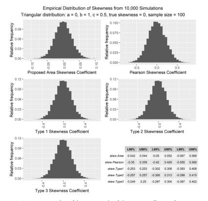
**Figure 15.** Histograms and confidence intervals of skewness coefficients from 10,000 simulations of n = 100 samples from Tr (0, 0.5, 1).
