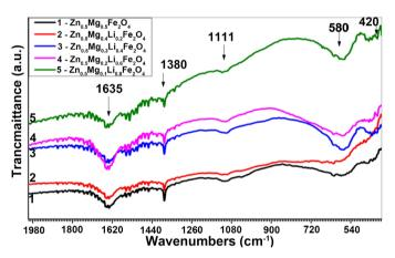
**Figure 2.** The Fourier Transform Infrared Spectrophotometer of Zn<sub>0.5</sub>Li<sub>2x</sub>Mg<sub>0.5-x</sub>Fe<sub>2</sub>O<sub>4</sub> samples.
