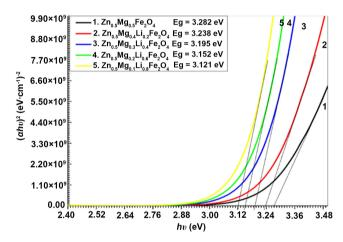
Figure 4. The optical energy bandgab of Zn<sub>0.5</sub>Li<sub>2x</sub>Mg<sub>0.5-x</sub>Fe<sub>2</sub>O<sub>4</sub> samples.
