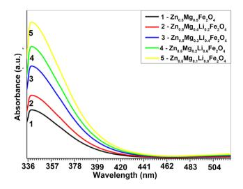
**Figure 3.** The relation between absorbance and wavelengths of Zn<sub>0.5</sub>Li<sub>2x</sub>Mg<sub>0.5-x</sub>Fe<sub>2</sub>O<sub>4</sub> samples.
