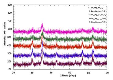
Figure 1. XRD spectrum of Zn<sub>0.5</sub>Li<sub>2x</sub>Mg<sub>0.5-x</sub>Fe<sub>2</sub>O<sub>4</sub> series.
