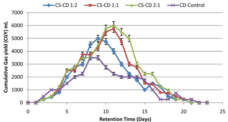
**Figure 5.** Progress curve showing the Daily Gas Yield (DGY) for the co-digestion of Corn Stalk (CS) and Cow Dung (CD) at different mixing ratios with a retention time of 24 days.
