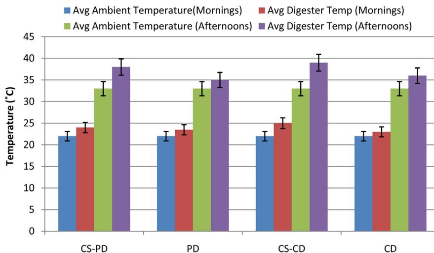
**Figure 7.** Measurement of Temperature from the co-digestion of Corn Stalk (CS) with Poultry Droppings (PD), Cow Dung (CD) at different mixing ratios. Note: \*Initial ambient temperature in the mornings and average ambient temperature between 11 am and 5 pm is  $35^{\circ}\text{C} \pm 2^{\circ}\text{C}$ . Initial average digester temperature was ambient temperature.
