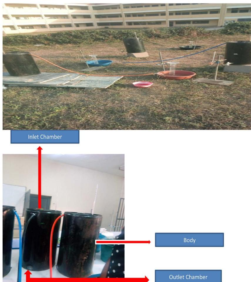
**Figure 1.** Experimental set up with 30 L bio-digester.
