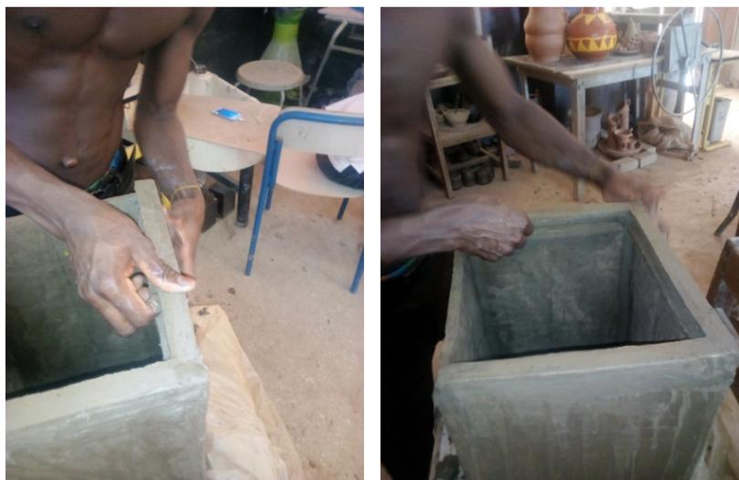
**Figure 12.** Constructing lids of container.
