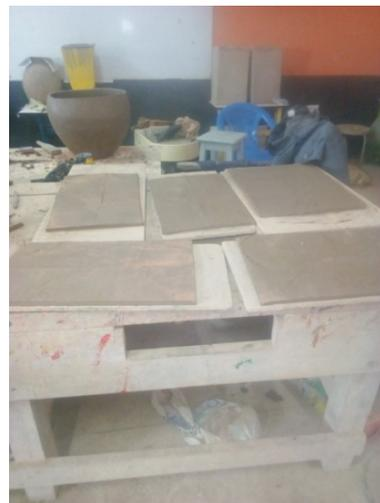
**Figure 8.** Drying of constructed slabs.
