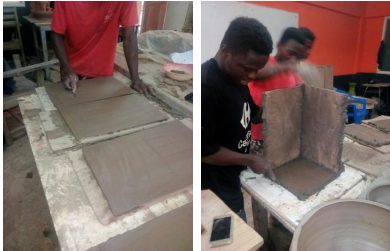
**Figure 10.** Applying slip and joining of parts of container.
