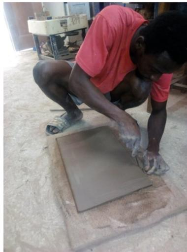
**Figure 7.** Cutting of slab into shape.
