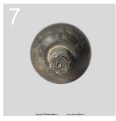
**Figure 9.** The mark on the head of pin in a ball bearing.
