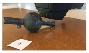
**Figure 12.** ELIO XRF portable system acquiring fluorescence spectrum from the ball bearing n.8.
