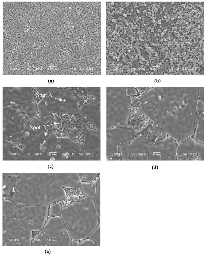
**Figure 3.** SEM micrographs of  $\text{Li}_2\text{ZnTi}_3\text{O}_8$  ceramics doped with different amounts of  $\text{V}_2\text{O}_5$  sintered at different temperatures; (a) 0 wt%,  $900^\circ\text{C}$ ; (b) 0.25 wt%,  $900^\circ\text{C}$ ; (c) 0.5 wt%,  $900^\circ\text{C}$ ; (d) 0.75 wt%,  $900^\circ\text{C}$ ; (e) 1 wt%,  $900^\circ\text{C}$ .
