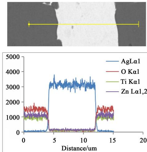
**Figure 7.** EDS line scanning of the  $\text{Li}_2\text{ZnTi}_3\text{O}_8$  ceramics co-fired with Ag.
