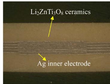
**Figure 6.** Optical microscopy of  $\text{Li}_2\text{ZnTi}_3\text{O}_8$  ceramics co-fired with Ag.
