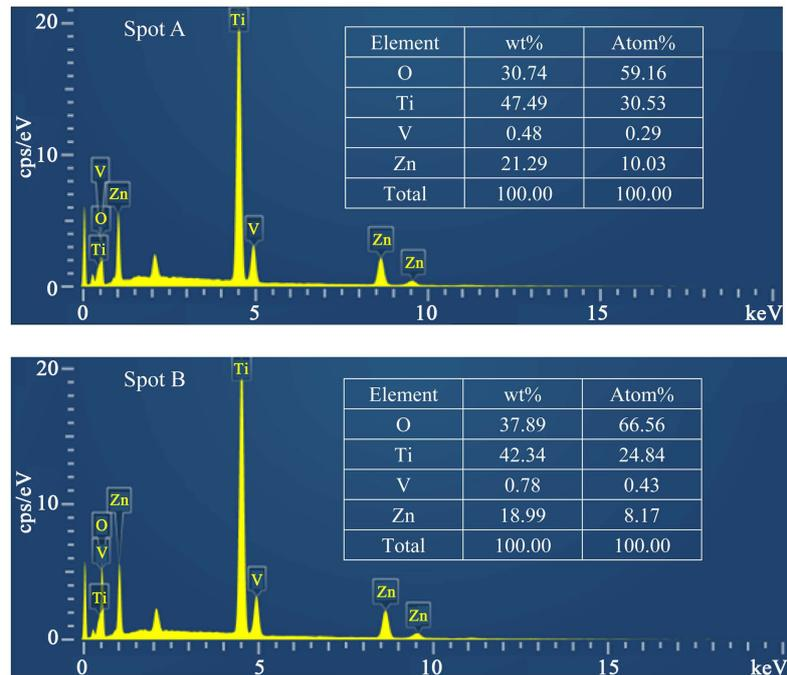
**Figure 4.** EDS analysis of  $\text{Li}_2\text{ZnTi}_3\text{O}_8$  ceramics added with 0.5 wt%  $\text{V}_2\text{O}_5$  and sintered at  $900^\circ\text{C}$  for 3 h.
