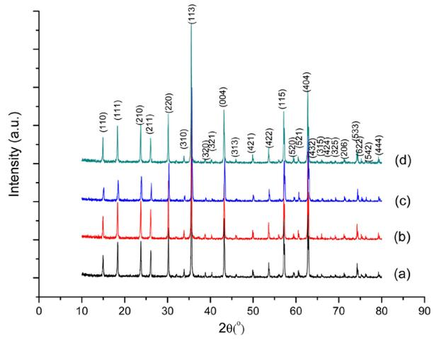
**Figure 2.** XRD patterns of  $\text{Li}_2\text{ZnTi}_3\text{O}_8$  ceramics doped with different amounts of  $\text{V}_2\text{O}_5$  and sintered at  $900^\circ\text{C}$ ; (a) 0.25 wt%; (b) 0.5 wt%; (c) 0.75 wt%; and (d) 1 wt%.
