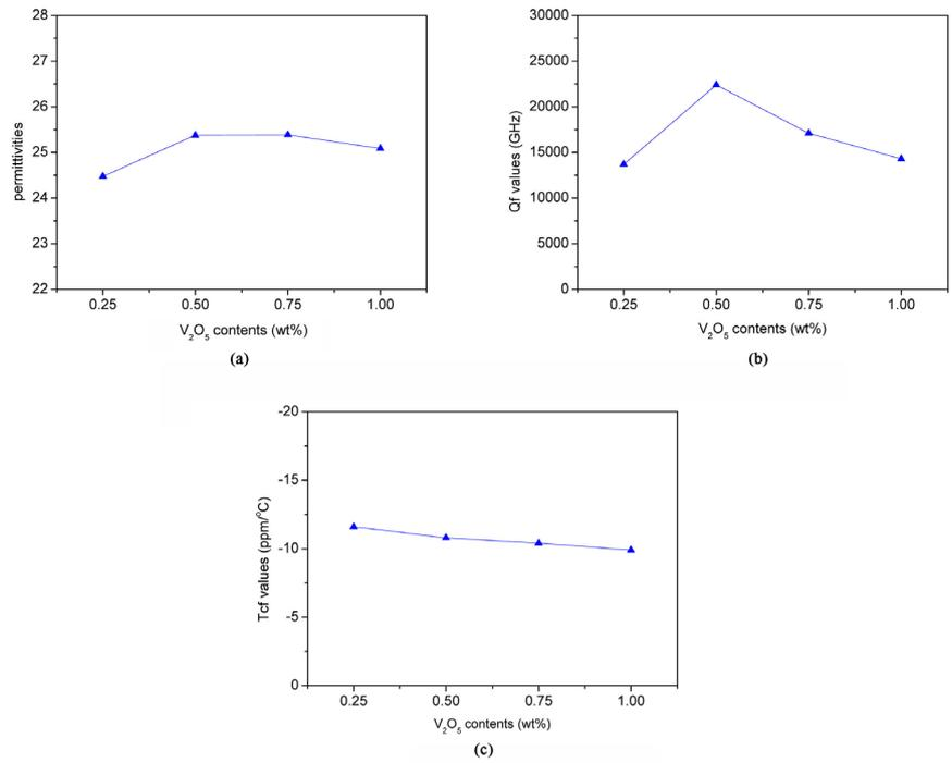
**Figure 5.** Microwave dielectric properties of  $\text{Li}_2\text{ZnTi}_3\text{O}_8$  ceramics as a function of  $\text{V}_2\text{O}_5$  addition content; (a) Relative permittivity; (b) Qf values; and (c)  $\tau_f$  values.
