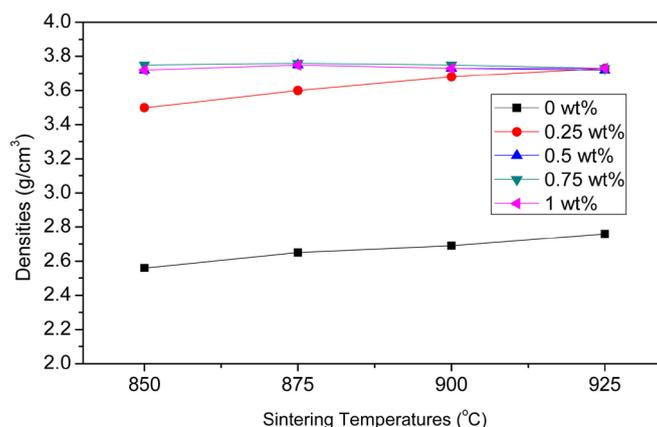
**Figure 1.** Densities of  $\text{Li}_2\text{ZnTi}_3\text{O}_8$  ceramics as a function of sintering temperatures and the  $\text{V}_2\text{O}_5$  addition contents.
