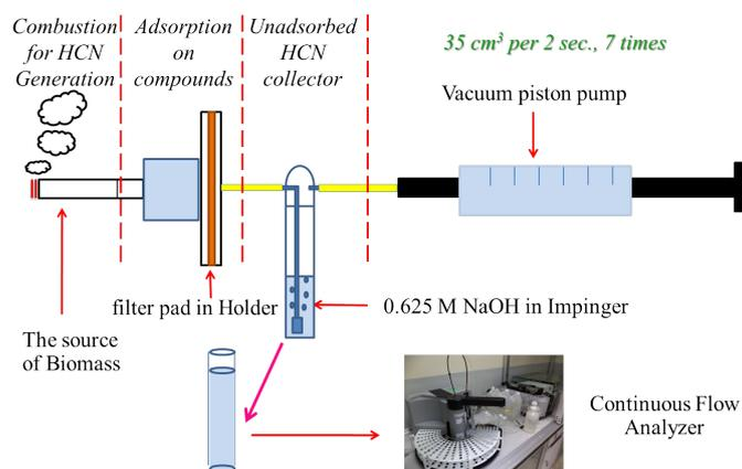
**Figure 1.** The experimental set for adsorption of hydrogen cyanide from combustion of dried stripes of tobacco leaves.
