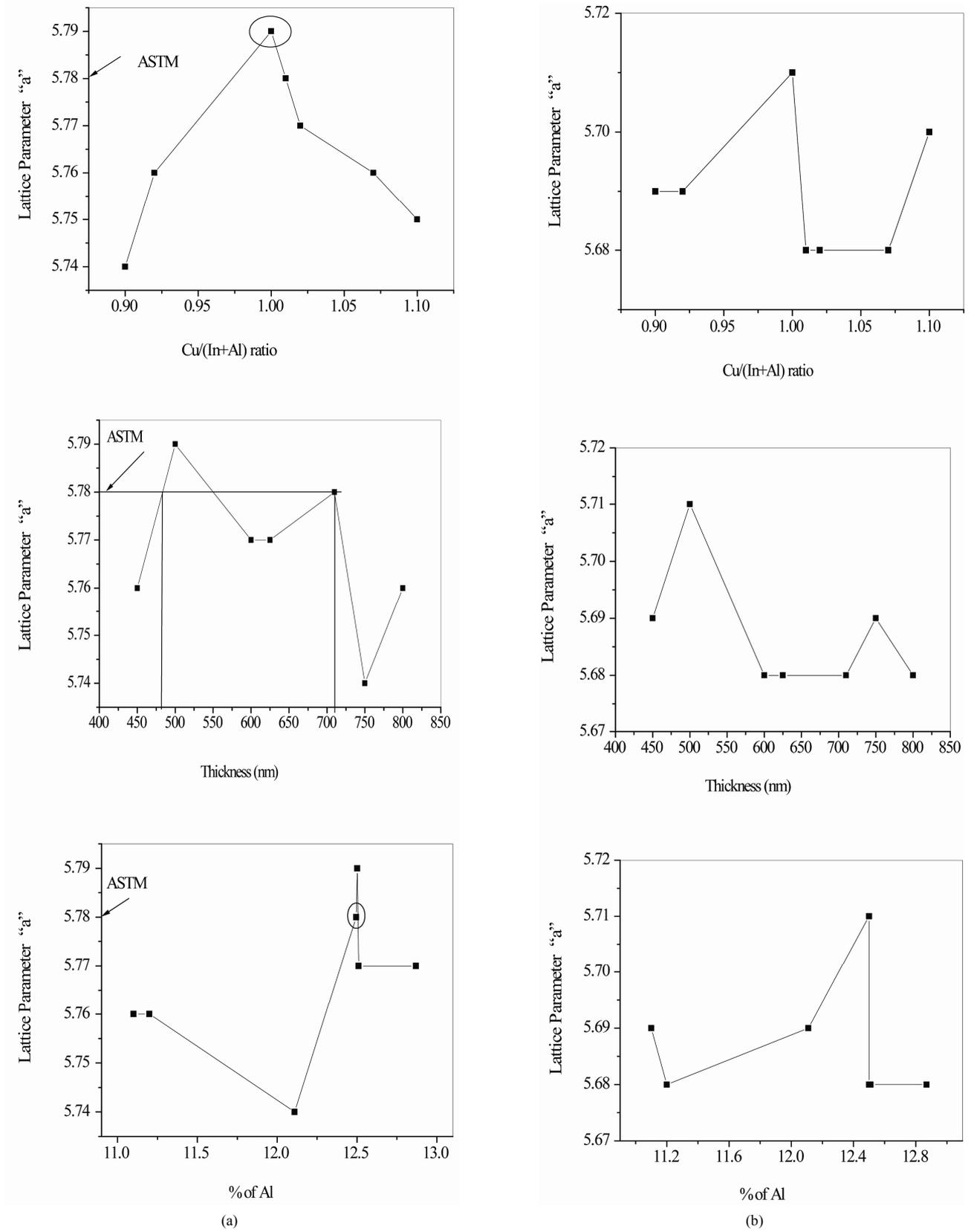
**Figure 2. Variation of f lattice parameter "a" [estimated from (a) XRD spectra; (b) EDAX spectra] with film parameters.**
