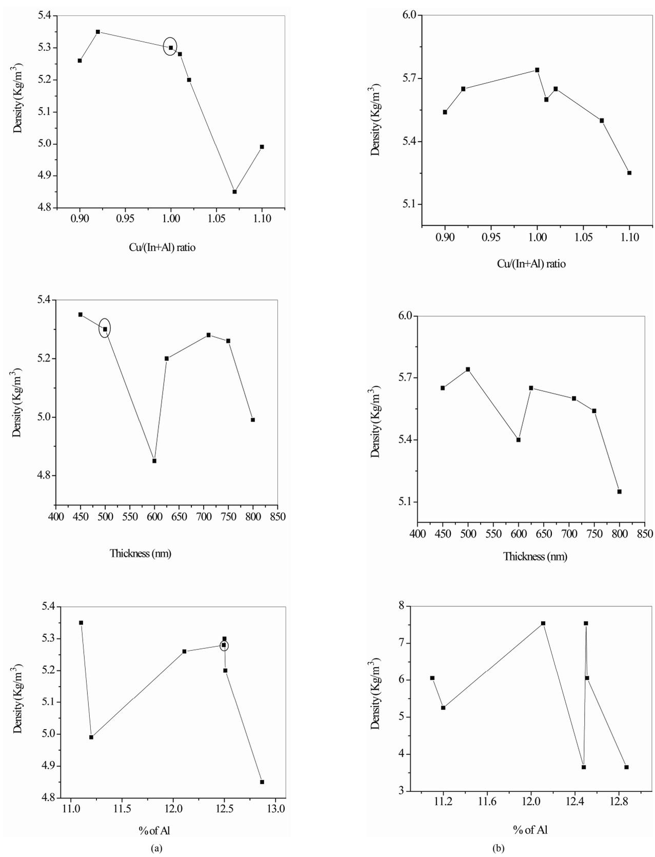
Figure 6. Variation of density [estimated from (a) XRD spectra; (b) EDAX spectra] with film parameters.
