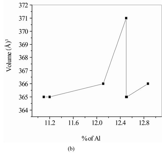
Figure 5. Variation of volume [estimated from (a) XRD; spectra (b) EDAX spectra] with film parameters.
