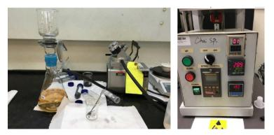
**Figure 2.** Synthesis  $rGO-TiO_2$  (S) via solvothermal method by using a Teflon-Lined autoclave.
