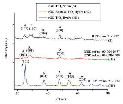
Figure 4. XRD patterns of rGO-TiO<sub>2</sub> (S), rGO-TiO<sub>2</sub> (H1) and rGO-Anatase TiO<sub>2</sub> (H2).
