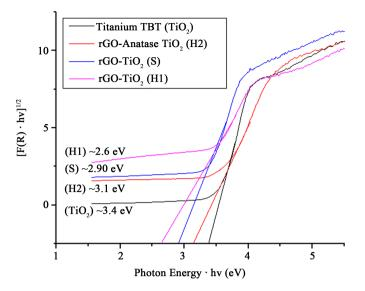
**Figure 7.** Kubelka-Munk function plot of titanium (TiO<sub>2</sub>), rGO-Anatase TiO<sub>2</sub> (H2), rGO-TiO<sub>2</sub> (S) and rGO-TiO<sub>2</sub> (H1).
