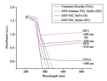
**Figure 6.** UV Vis diffuse reflectance spectra of titanium (TiO<sub>2</sub>), rGO-Anatase TiO<sub>2</sub> (H2), rGO-TiO<sub>2</sub> (S) and rGO-TiO<sub>2</sub> (H1).
