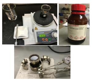
**Figure 3.** Synthesis  $rGO-TiO_2$  (H1) and  $rGO-TiO_2$  (H2) via hydrothermal method by using a Teflon-Lined autoclave.
