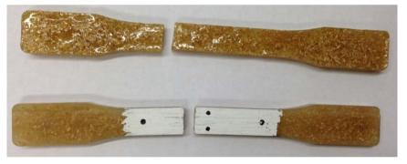
**Figure 5.** RHP-Epoxy 0.30 Volume Fraction Samples—Premilled (Top) and Milled (Bottom).
