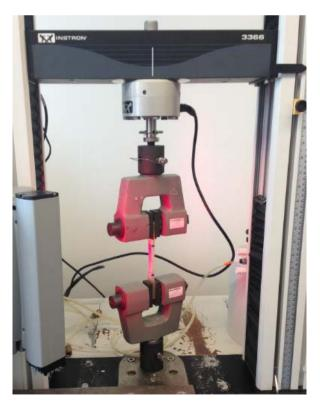
Figure 7. Instron 3366 10 kN dual column testing systems with a video extensometer.
