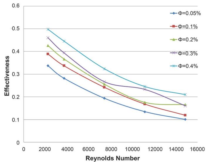
**Figure 6.** Effectiveness vs Reynolds Number at 5 m/s air velocity.
