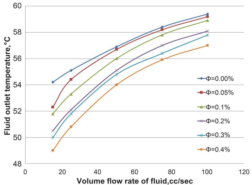
**Figure 3.** Fluid outlet temperature vs Volume flow rate of fluid.
