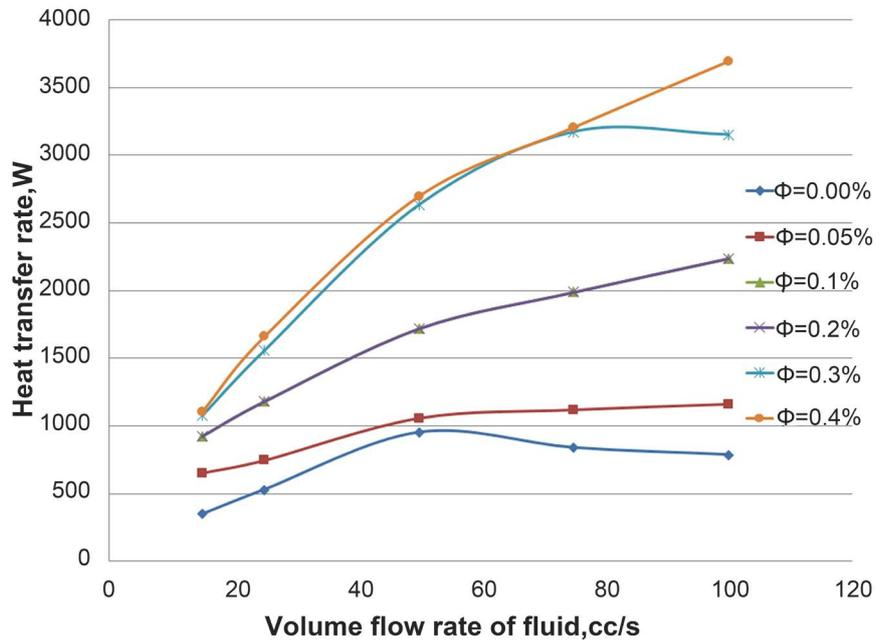
Figure 4. Heat Transfer rate vs Volume flow rate of fluid.
