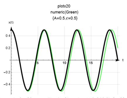
**Figure 5.** Display of the numeric (Green) and Power Series Method (Black) of modified Duffing equation with  $\epsilon x^5(t)$ ,  $\{A, \epsilon\} = \{0.5, 0.5\}$  with N = 20.
