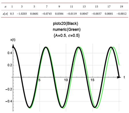
**Figure 4.** Display of the numeric (Green) and Power Series Method (Black) of modified Duffing equation with  $\epsilon x^4(t)$ ,  $\{A, \epsilon\} = \{0.5, 0.5\}$  for N = 20.
