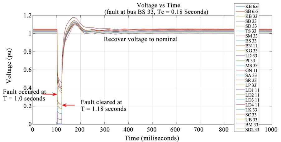
Figure 9. Voltage vs Time when faulted at bus BS\_33.
