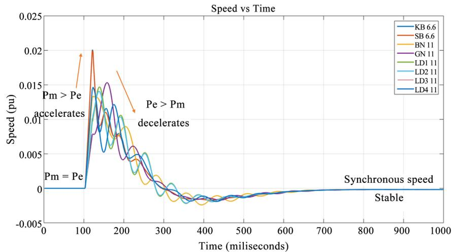
Figure 4. Impulse response of speed vs time for machines.
