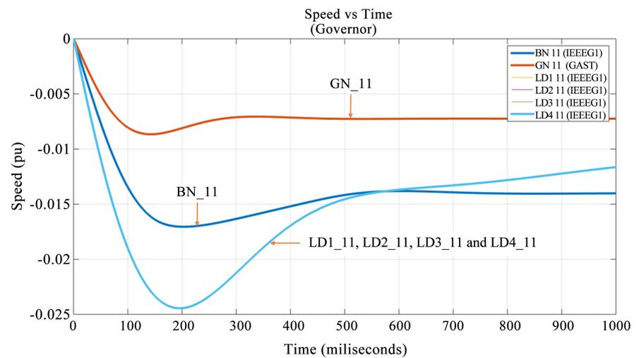
Figure 7. Step response of speed vs time for governors.
