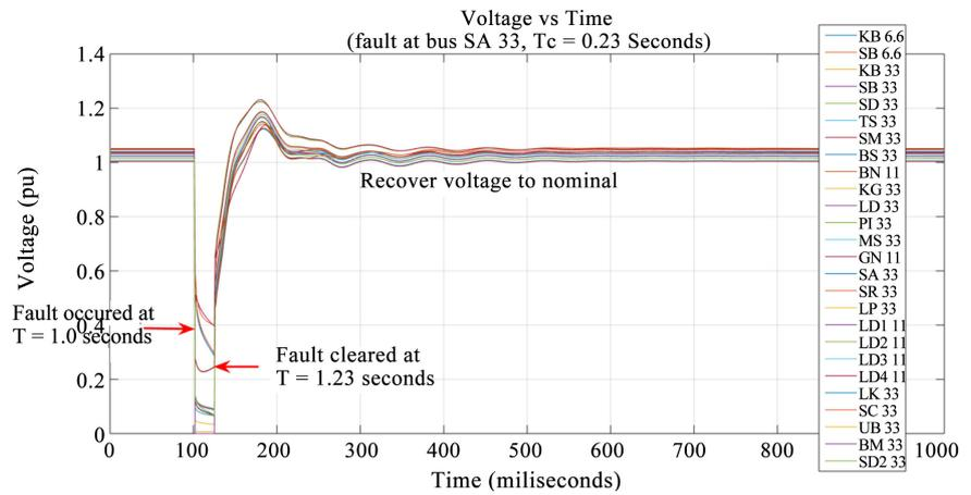
**Figure 10.** Voltage vs Time when faulted at bus SA<sub>33</sub>.
