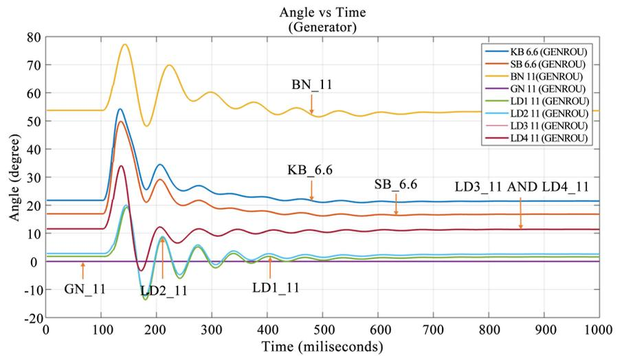
Figure 3. Swing rotor angle vs time for generators.
