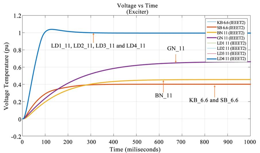
Figure 6. Terminal voltage vs time for exciters.
