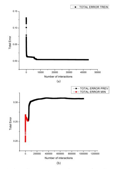
**Figure 13.** Total network training error interrupted at minimum data prediction error. (a) Total network training error; (b) Total data prediction error.
