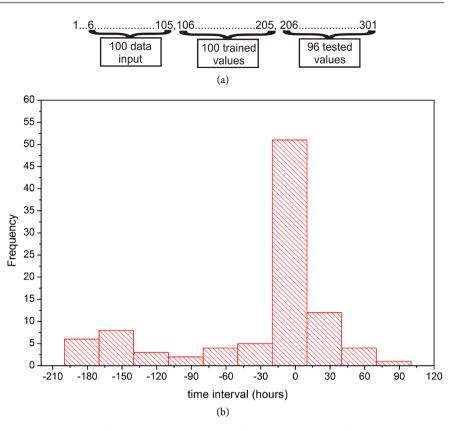
**Figure 10.** Data Shift Scheme and Histogram of the values tested after the training. (a) Scheme of the displacement of 5; (b) Histogram of the difference between real and network values for a 5 data shift.
