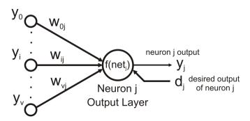
**Figure 5.** Output neuron *j*. The inputs are the activations of the neurons of the previous layer connected to the output.  $y_j$  represents the output generated by the network and  $d_j$  represents the desired output of neuron *j*.
