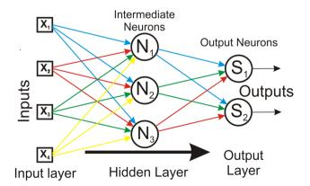
**Figure 3.** Illustration of a multilayer neural network structure.  $X_i$  are input data,  $N_i$  are intermediate layer neurons, and  $S_i$  are neurons of the output layer. The connections between the layers are made by the weights.
