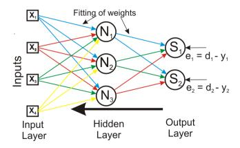
**Figure 4.** Illustration of the backpropagation of the error signals in the neural network.  $e_i$  represents the error signal obtained between the desired output and the output of the network and which will be propagated in the network to adjust the weights.
