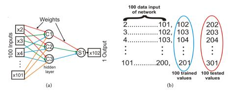
**Figure 9.** Scheme of the neural network used and how training and actual data were performed. (a) Schematic of the neural network used; (b) Training scheme in the training of the real data.
