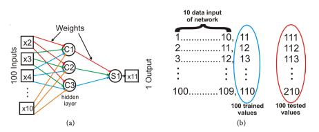
**Figure 7.** Schematic of neural network used and how training and actual data were performed. (a) Schematic of neural network used; (b) Training scheme and training of actual data.
