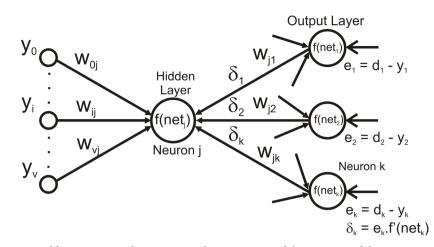
**Figure 6.** Hidden neuron *j*. The inputs are the activations of the neurons of the previous layer connected to the hidden neuron, being this neuron connected to the output neurons.  $\delta_k$  represents the local gradient of the output neurons. When we have only one hidden layer, the inputs of these neurons are the data input.
