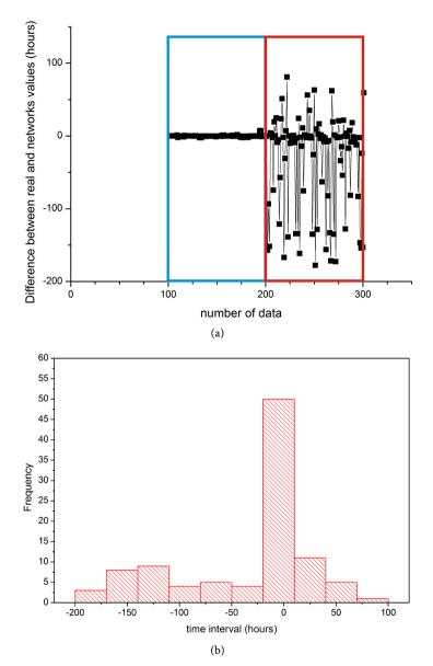
**Figure 8.** Scheme of the data trained and tested with histogram of the data tested. (a) Schematic of the trained data and tested; (b) Histogram of the difference between the data tested and the actual and estimated values.
