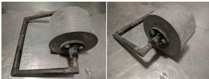
Figure 2. Hand-held roller for compacting pervious concrete cylinders.
