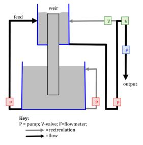
Figure 1. Schematic representation of the sediment dosing system.
