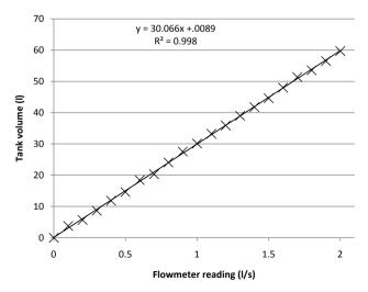
Figure 3. Calibration curve for flowmeter.
