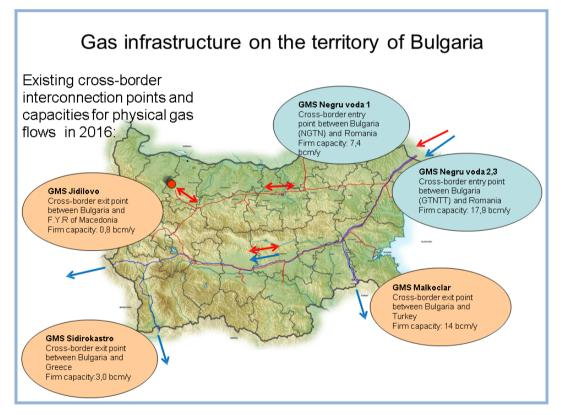
Figure 3. Bulgartransgaz EAD network development plans [10].
