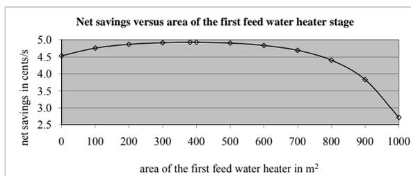
**Figure 3. Variation of total cost versus area of the first feed water heater.**
