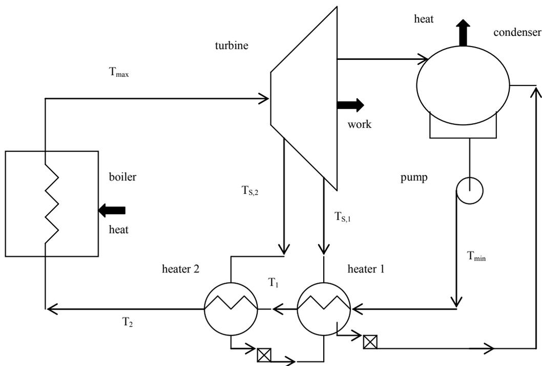
Figure 1. Schematic figure of a typical thermal power plant that employs two closed feed water heater.
