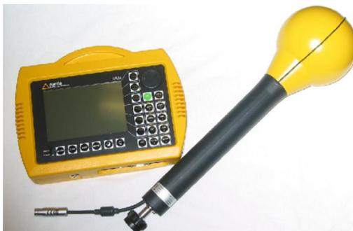
Figure 2. Narda narrowband field meter (SRM3000).
