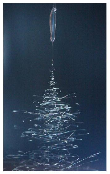
Figure 1. Ideal electrospinning process.
