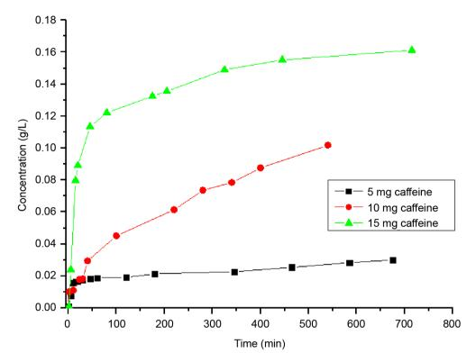
Figure 4. Kinetics of caffeine delivery from PLLA membrane obtained after 10 minutes of electrospinning.
