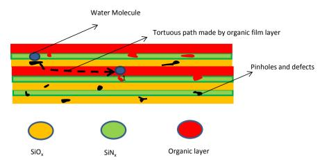
Figure 6. Tortuous path made by organic layer between two inorganic layers.
