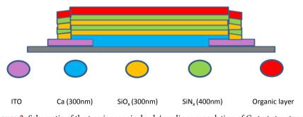
Figure 3. Schematic of the two inorganic dyads/acrylic encapsulation of Ca test structure.
